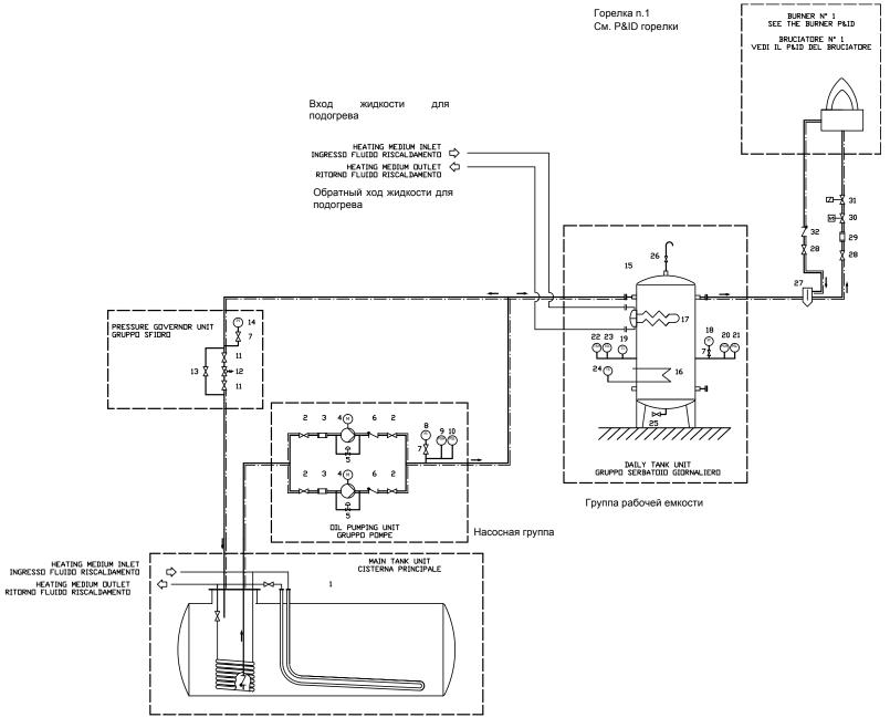
Fig. 14 - 3ID0023 v2 - Hydraulic diagram - Single burner configuration
