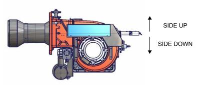
Burner is designed to operate with horizontal flame axis. Set the upper side of the burner flange in a horizontal position, in order to obtain the correct inclination of the pre-heating tank. For different installations, please contact the Technical Department.
