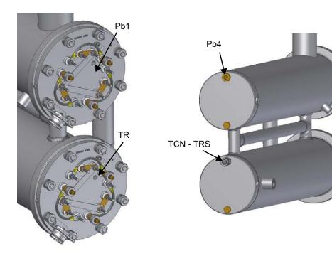
Fig. 18 - Probe connections (Danfoss MCX)
