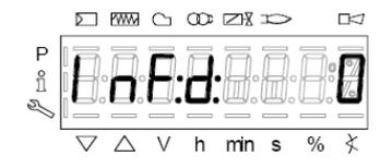
To reset, press InFo for a second. Record the codes and check the Error List to find the type of faults.
