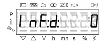
To reset, press InFo for a second. Record the codes and check the Error List to find the type of faults.
