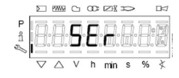
The service level shows all the information about flame intensity, actuators position, number and lock codes:
