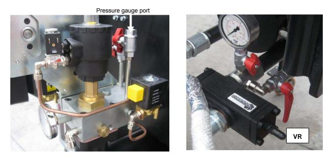
6 Set the atomisation air according to the data in the nozze diagram attached, by means of the RB knob (see picture).
