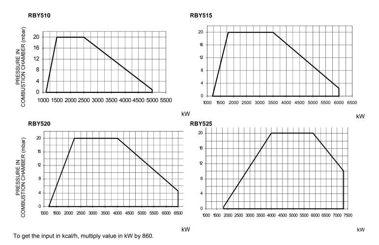
Data are referred to standard conditions: atmospheric pressure at 1013mbar, ambient temperature at 15°C.
