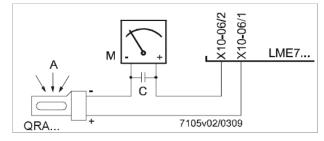
Fig. 15: Detection by photocell QRA..
