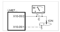
Fig. 14: Detection by electrode
