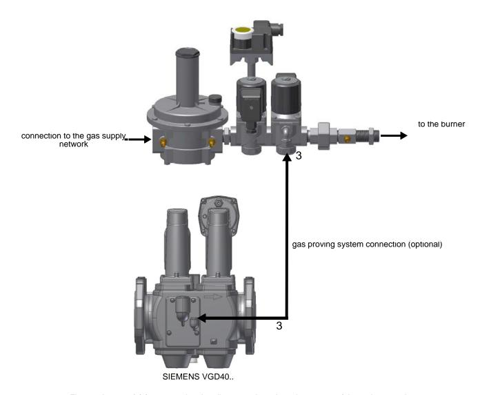
Fig. 5 - pipe port (3) for connecting the pilot gas train to the valves group of the main gas train
