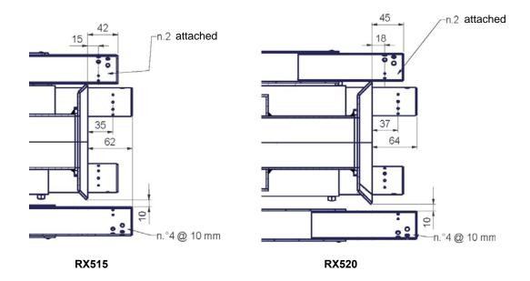
The smallest holes (pilot holes) are directed towards the flame axis while the biggest ones (main holes) are directed outwards. As for a finest adjustment in the plant, please contact the Technical service.
