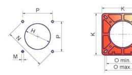
boiler recommended drilling template and burner flange
