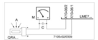
Fig. 15: Detection by photocell QRA..
