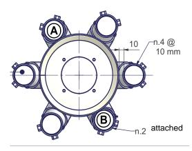
There are six nozzles: two are in touch with the diffuser and are diametrically opposite, four are placed at 10mm from the diffuser edge (see picture above).
