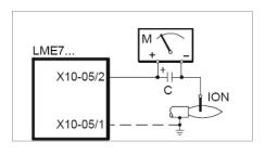
Fig. 14: Detection by electrode
