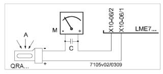
Fig. 18: Detection by photocell QRA..
