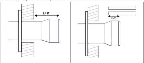
The length of the blast tubes does not always allow this requirement to be met, and thus it may be necessary to use a suitably-sized spacer to move the burner backwards or to design a blast tube tha suites the utilisation (please, contact the manifacturer).
