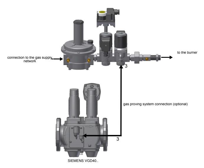
Fig. 12 - pipe port (3) for connecting the pilot gas train to the valves group of the main gas train
