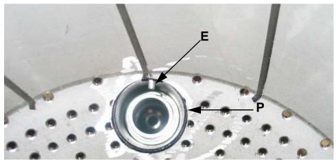
Fig. 15 - Detailed view of the diffuser with pilot (P) and ignition elecctrode (E)
