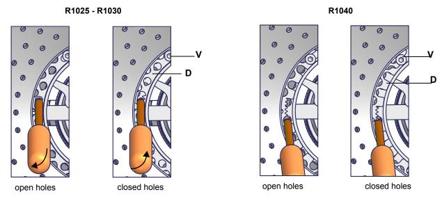
The adjusting plate correct position must be regulated in the plant during the commissioning. The factory setting depends on the type of fuel for which the burner is designed:
