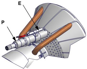
Fig. 16 - Detailed view of the combustion head with pilot (P) and ignition elecctrode (E)
