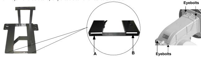
The burner is provided with eyebolts, for handling operations.
