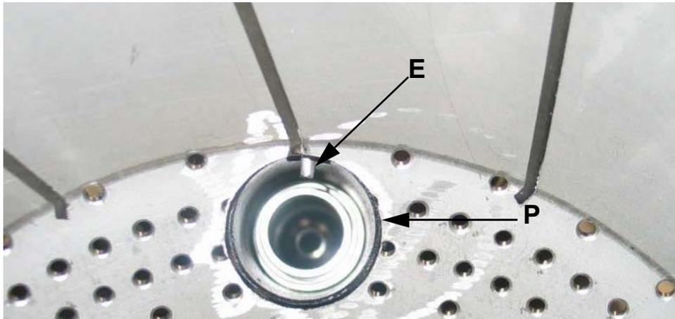
Fig. 15 - Detailed view of the diffuser with pilot (P) and ignition electrode (E)
