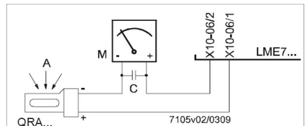
Fig. 18: Detection by photocell QRA..
