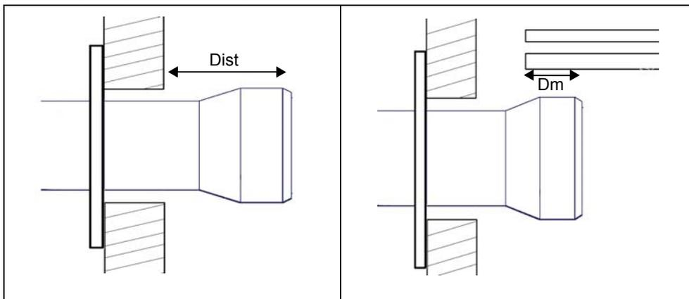
The length of the blast tubes does not always allow this requirement to be met, and thus it may be necessary to use a suitably-sized spacer to move the burner backwards or to design a blast tube that suits the utilisation (please, contact the manufacturer).
