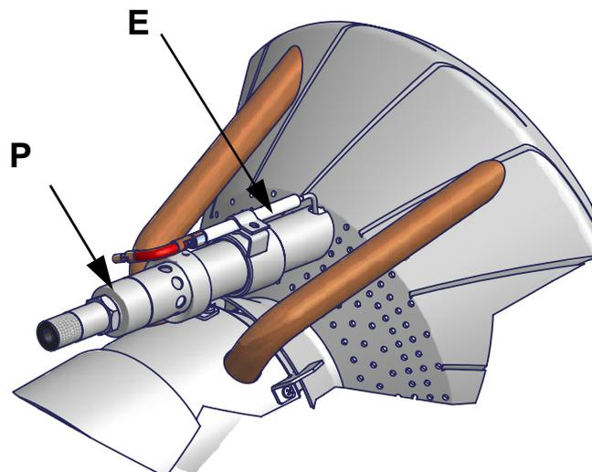
Fig. 16 - Detailed view of the combustion head with pilot (P) and ignition electrode (E)
