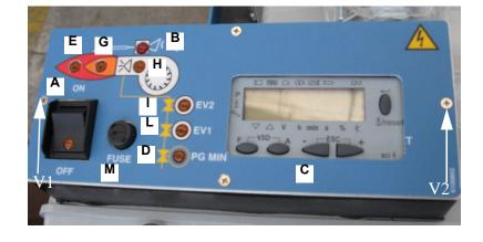
Fig. 46 - Burner's control panel
