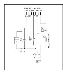
Fig. 35 - 7-pins connector
