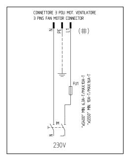
Fig. 40 - Electric motor's 3-pin connector for NG/LG/NGXG400
