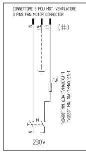
Fig. 38Electric motor's 3-pin connector for NG/LG/NGX400
