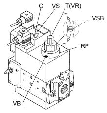
Go on adjusting air and gas flow rates: check, continuosly, the flue gas analisys, as to avoid combustion with little air; dose the air according to the gas flow rate change following the steps quoted below;
