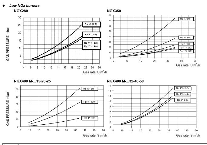
Caution: the gas rate value is quoted on the x-axis, the related network pressure is quoted on the y-axis (pressure value in the combustion chamber is not included). To know the minimum pressure at the gas train inlet, necessary to get the requested gas rate, add the pressure value in the combustion chamber to the value read on the y-axis.
