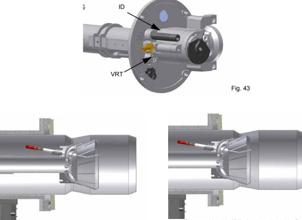
Fig. 44 - Head in "fully-ahead position"
