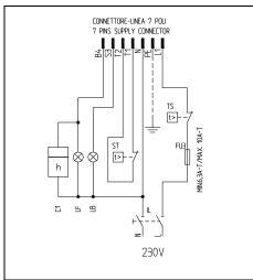
Fig. 39 - 7-pin connector
