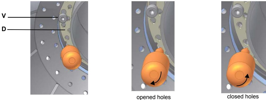
The adjusting plate correct position must be regulated in the plant during the commissioning.
