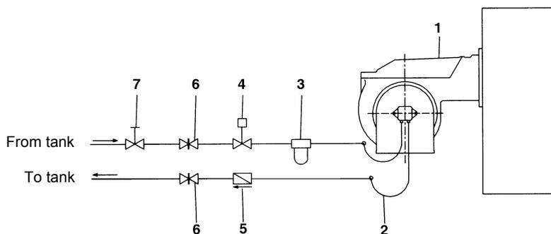
Fig. 16 - Double-pipe system
