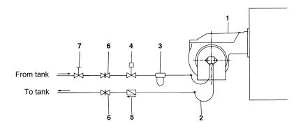
Fig. 16 - Double-pipe system
