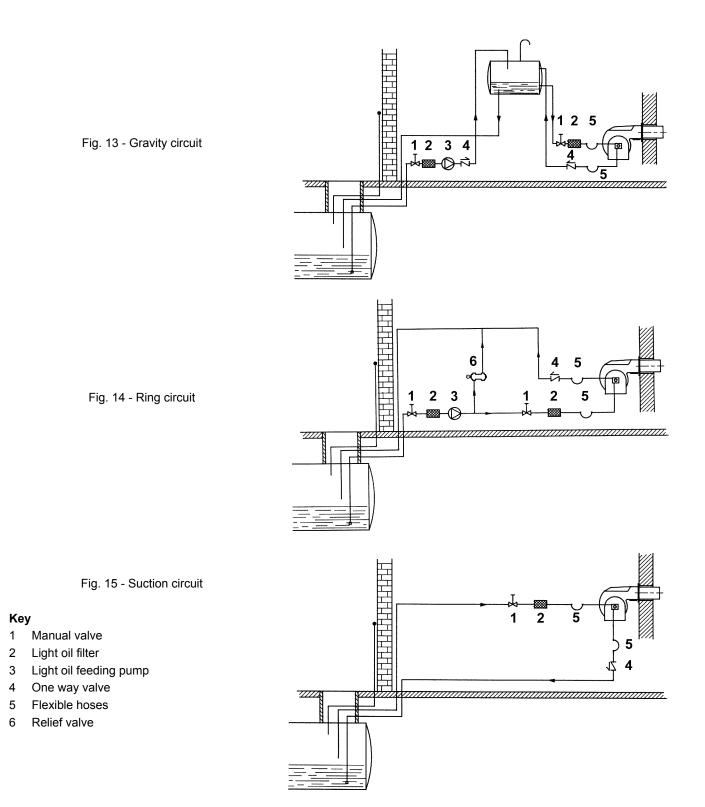
**NOTE:** in plants where gravity or ring feed systems are provided, install an automatic interception device.
