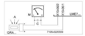
Fig. 24: Detection by photocell QRA..
