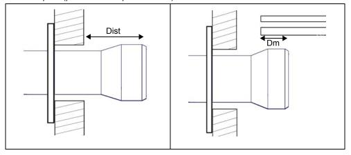
The length of the blast tubes does not always allow this requirement to be met, and thus it may be necessary to use a suitably-sized
