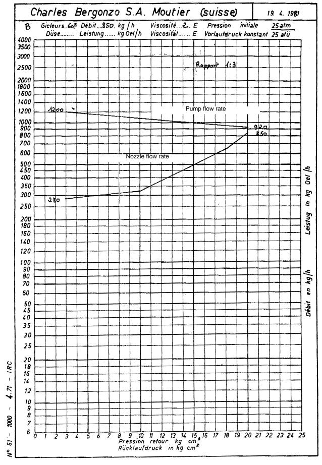
Fig. 19 - Bergonzo B nozzle - example with 850kg/h nozzle
