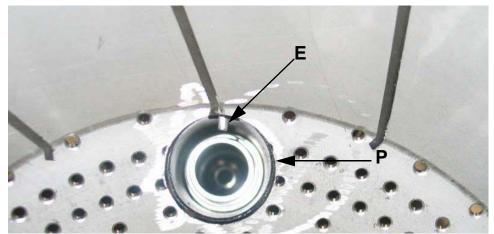
Fig. 24 - Detailed view of the diffuser with pilot (P) and ignition elecctrode (E)
