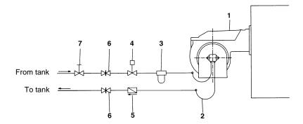
Fig. 16 - Double-pipe system
