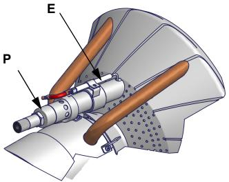
Fig. 25 - Detailed view of the combustion head with pilot (P) and ignition elecctrode (E)
