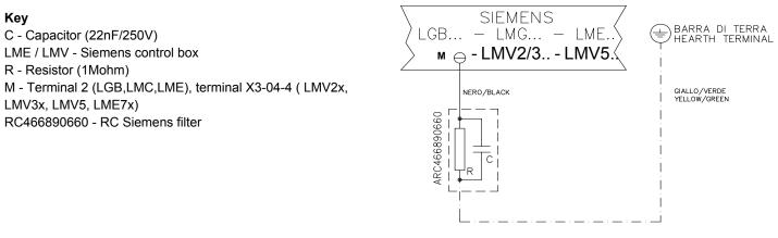
For LMV5 control box, please refer to the clabeling recommendations available on the Siemens CD attached to the burner
