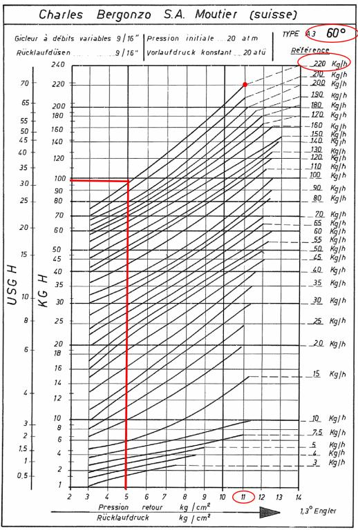
**Example:** if a 220kg/h flow rate BERGONZO nozzle is provided, set the return pressure at 11bar, supply at 20bar on the delivery to get a 220kg/h flow rate. If the return pressure needed is 5bar, instead, act on the **V** adjusting screw on the pressure regulator (see next paragraph). The flow rate will then be about 95kg/h (see the example showed on the Bergonzo diagram).
