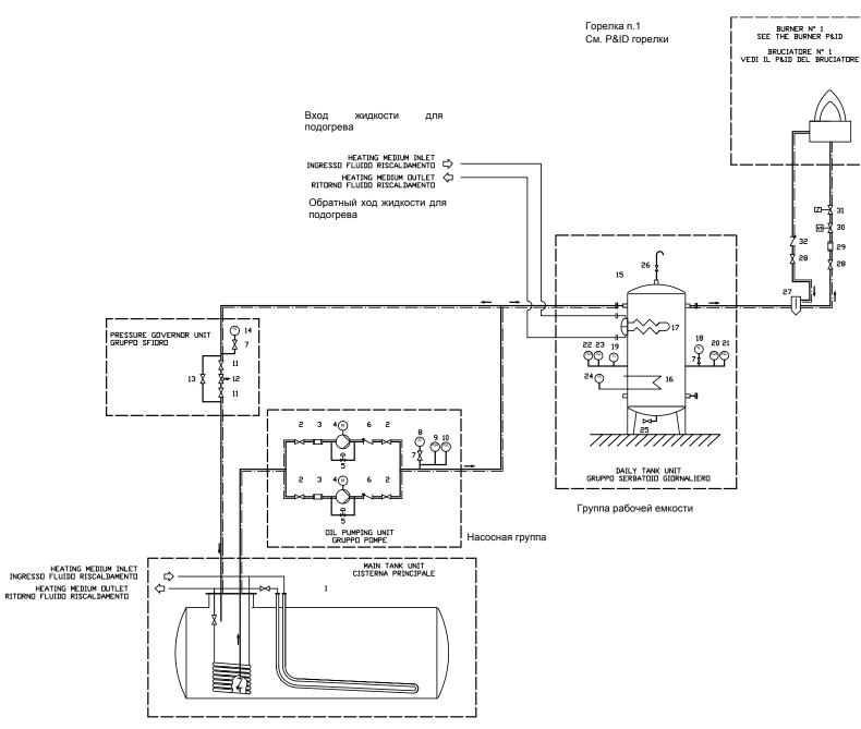
Fig. 18 - 3ID0023 v2 - Hydraulic diagram - Single burner configuration
