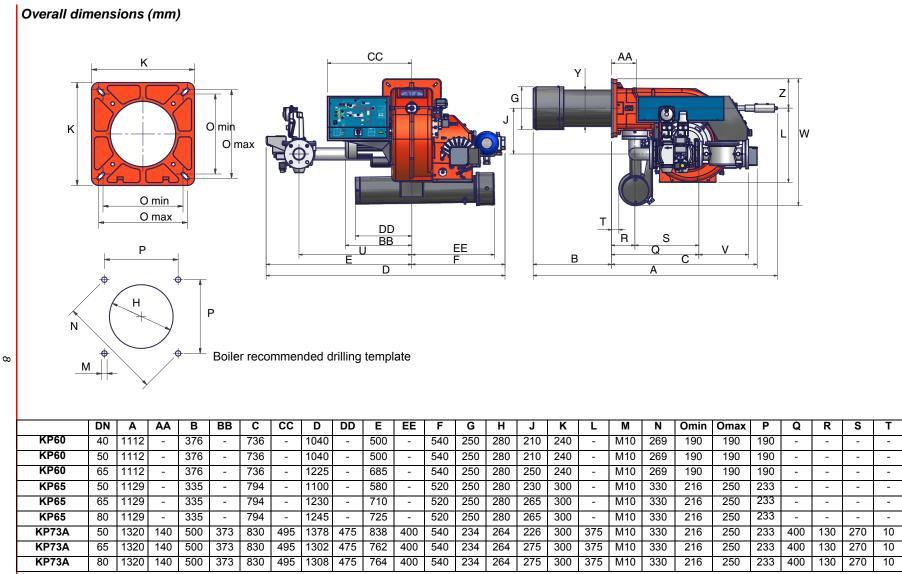
NOTE: the overall dimensions are referred to burners provided with Siemens VGD valves.
