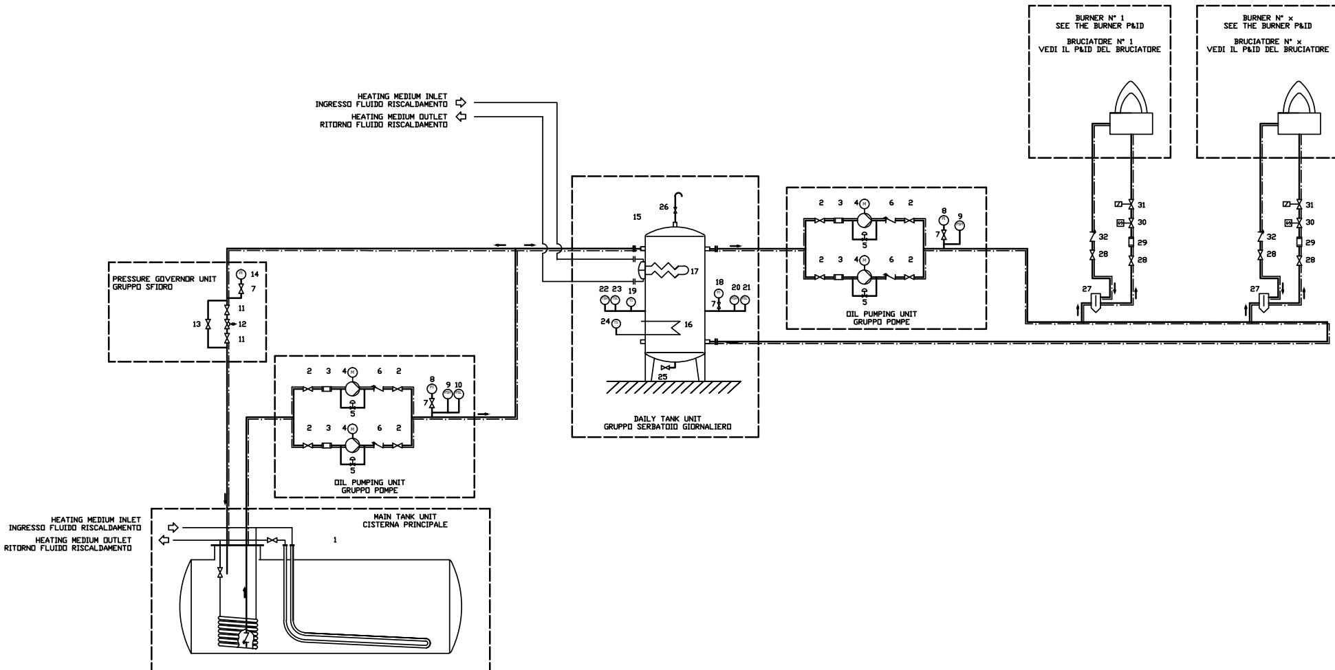
Fig. 17 - 3ID00014 v2 Hydraulic diagram - Two or more burners configuration
