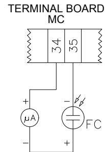
Fig. 37: Detection by photocell QRA..
