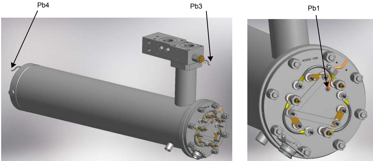
Fig. 29 - Probe connections (Danfoss MCX)
