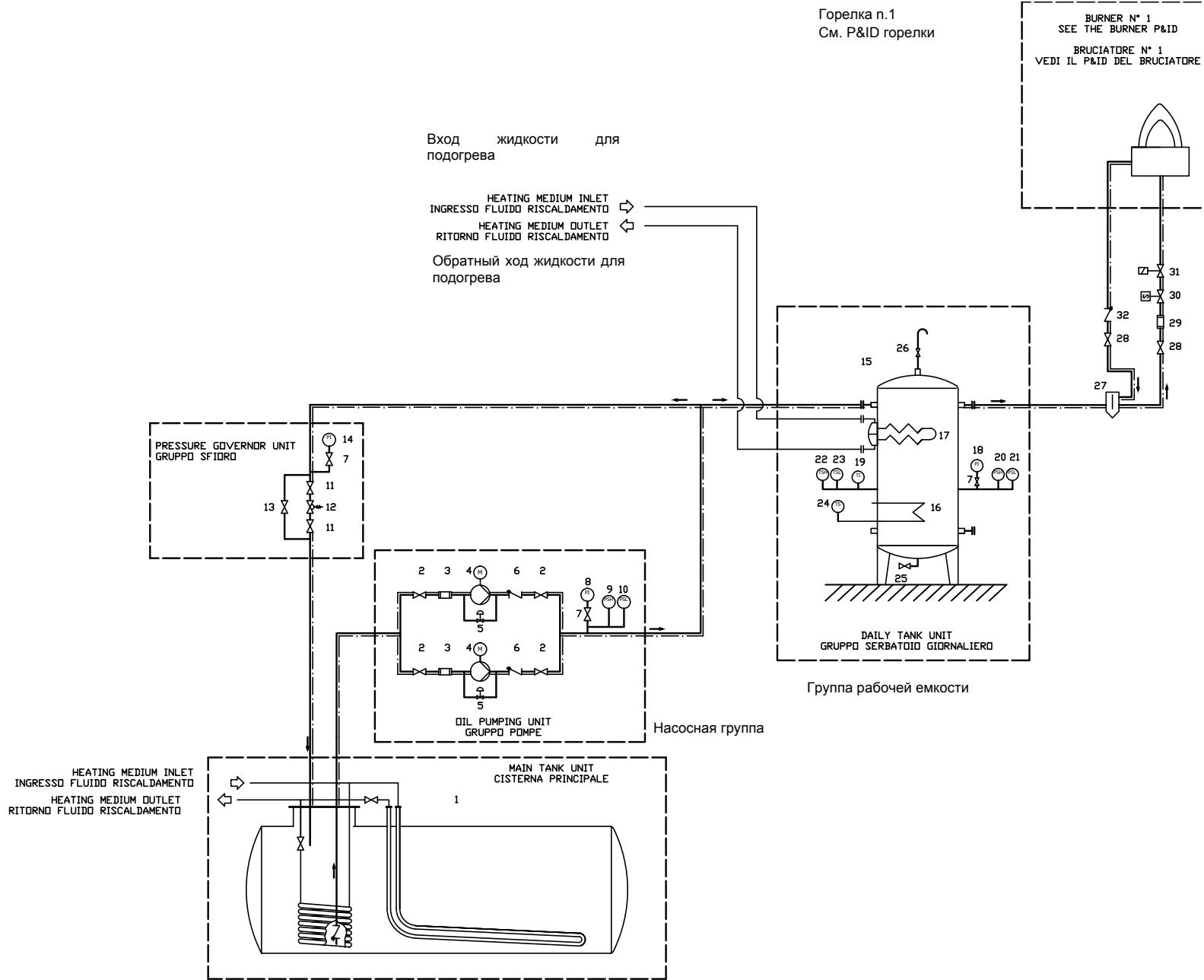
Fig. 18 - 3ID0023 v2 - Hydraulic diagram - Single burner configuration
