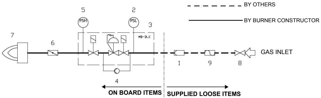
Gas train with valves group VGD with built-in gas pressure governor + gas proving system VPS504
