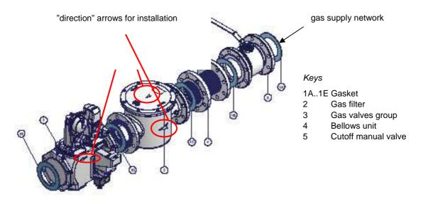
Fig. 4 - Example for gas train
