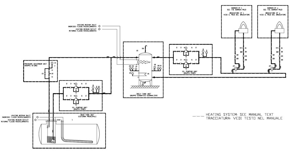
Fig. 11 - Two or more burners configuration
