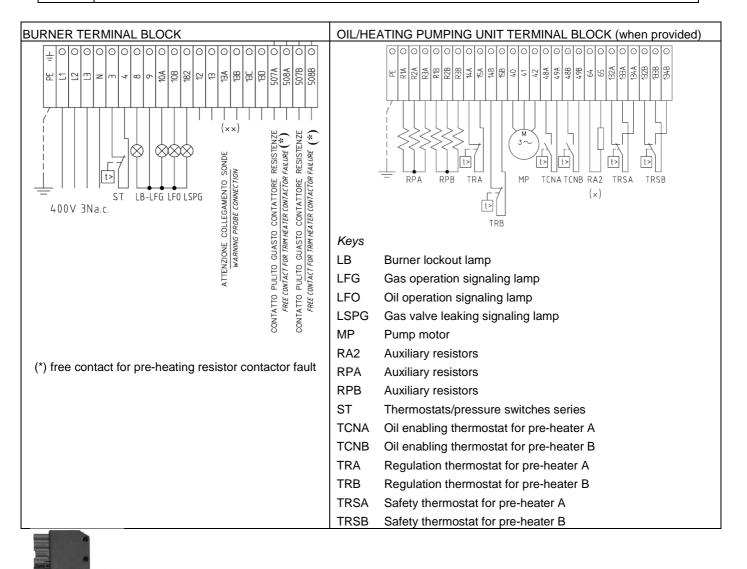
Probes connections by means of the 7-pin plug (see picture) - see wiring diagrams for connections.
