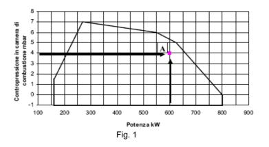
Data are referred to standard conditions (atmospheric pressure at 1013mbar, ambient temperature at 15°C).
