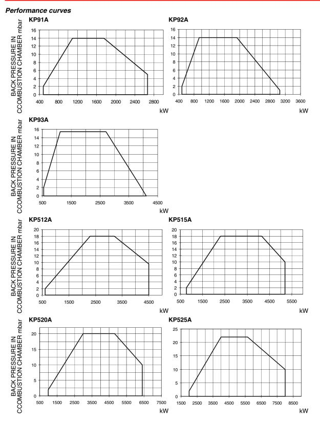
To get the input in kcal/h, multiply value in kW by 860. Data are referred to standard conditions: atmospheric pressure at 1013mbar, ambient temperature at 15°C.
