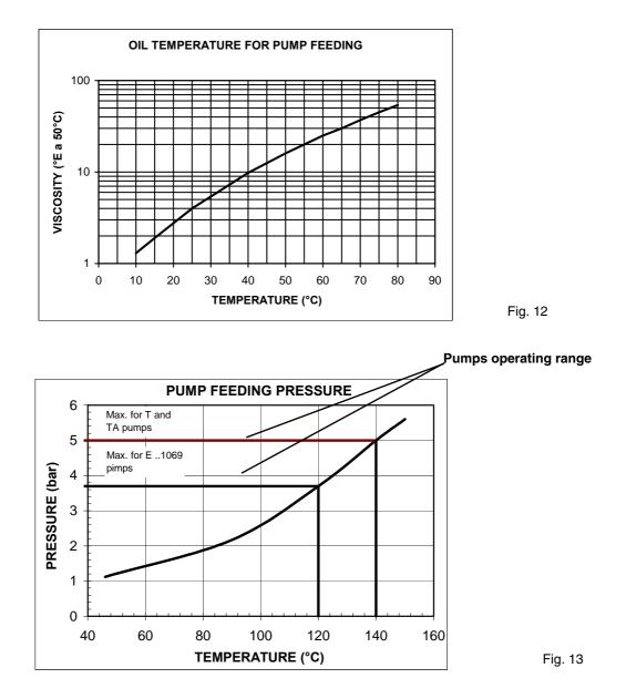
The use of heavy oil forces to feed the burner to a pressure strictly related to the oil temperature. This avoids damage to the pump caused by gassification.
