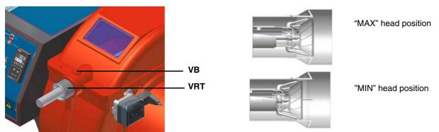
Attention! if it is necessary to change the head position, repeat the air and gas adjustments described above.
