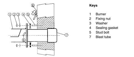
Set the upper side of the burner flange in a horizontal position, in order to obtain the correct inclination of the pre-heating tank.
